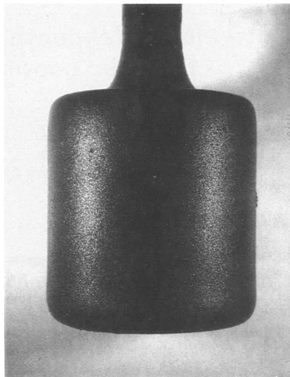
Figure 1 A photograph of one of the samples used in this study for the EIS measurements. The diameter of the sample is 10 mm.
